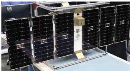
Figure 3.5a. One of the eight CYGNSS observatories prior to integration with the deployment module.
