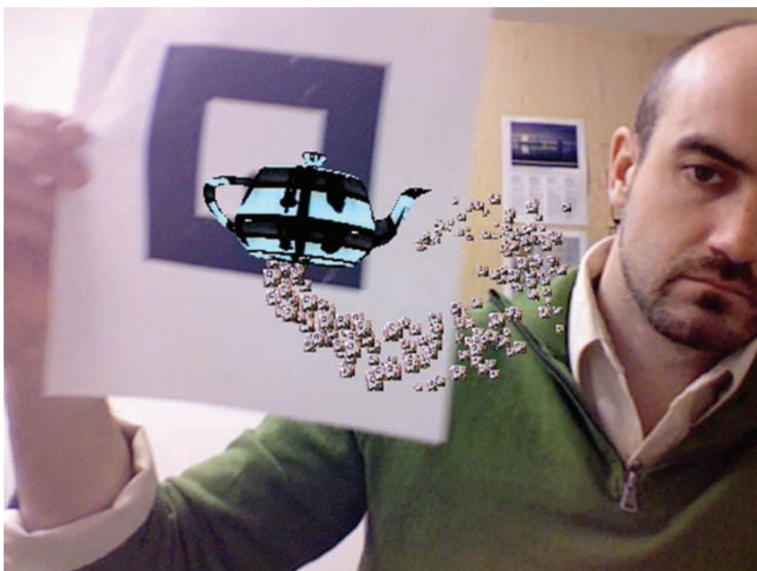
Figure 8.1. Test cube and marker outline superimposed on FLARToolkit marker.
